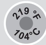
Limit temperature NOT exceeded
