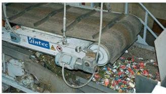
• **Overband Covers Belts:** Belts with these covers incorporate magnetic separators. They are made to order, according to the working conditions of each line.
