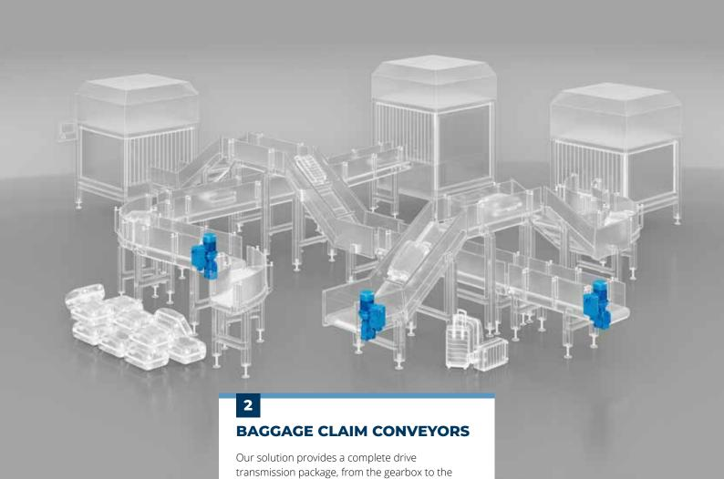
For baggage claim conveyors, our range is based on bevel gearboxes, always in combination with our IE3 electric motor and decentralized inverters. In this kind of applications where high efficiency is required, we can offer our synchronous reluctance motor with IE4 efficiency.
