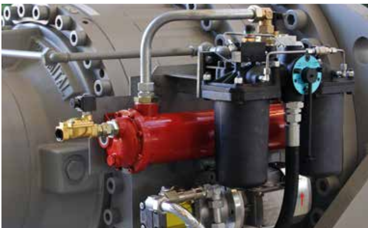
SPECIAL COOLING UNIT ON BOARD
