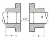
Dimension Y must be equal to or greater than Dimension X for clearance fits, or greater than Dimension X times .75 for interference fits. Example:  $X = 4^{\circ\circ}$ ; the Y must be 4° or more for clearance fits or 3" or more for interference fits.
