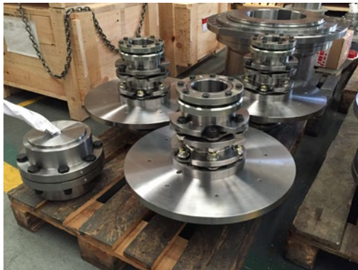
Disc pack configuration with brake disc.
