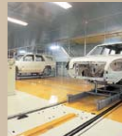
Conveyance System for Automobile Painting Lines
