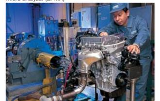
Testing a timing chain drive system
