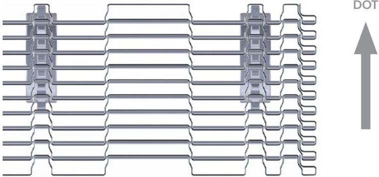
The sprockets of the PacTitan Pro™ should engage the belt within the narrower drive lane openings. The sprocket teeth should directly contact the rod surface within the openings (not the flat of the picket). The main engagement between the sprocket and belt edges is at the third opening in the picket, not to include the rectangular opening where the end of the rod is retained.
