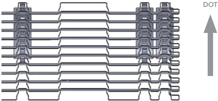
Under certain conditions, it may be desirable or advantageous to place additional sprockets at the extreme outer belt openings. This placement should only be used for heavily-loaded application conditions or as recommended by our Application Engineering team.
