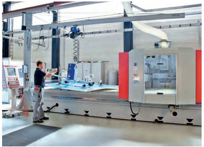
Aluminum column mounted jib crane with vacuum lifting device VacuMaster Comfort during loading of a CNC machining center
