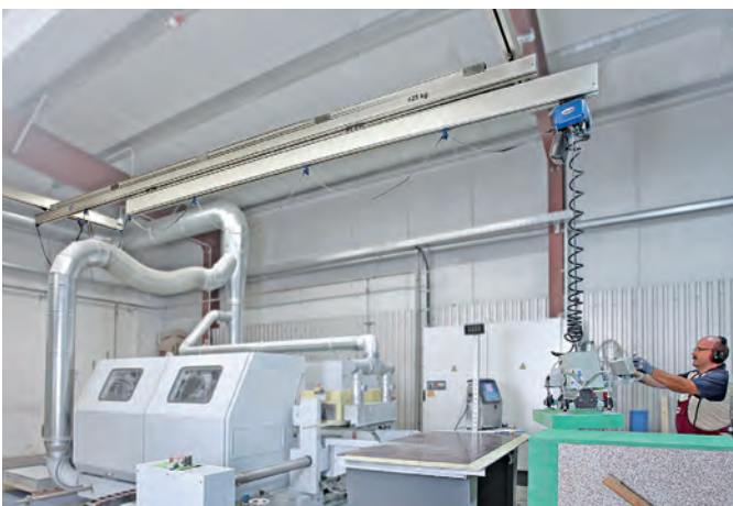
Aluminum single bridge crane system with telescopic jib and vacuum lifting device VacuMaster Comfort handling plastic sheets
