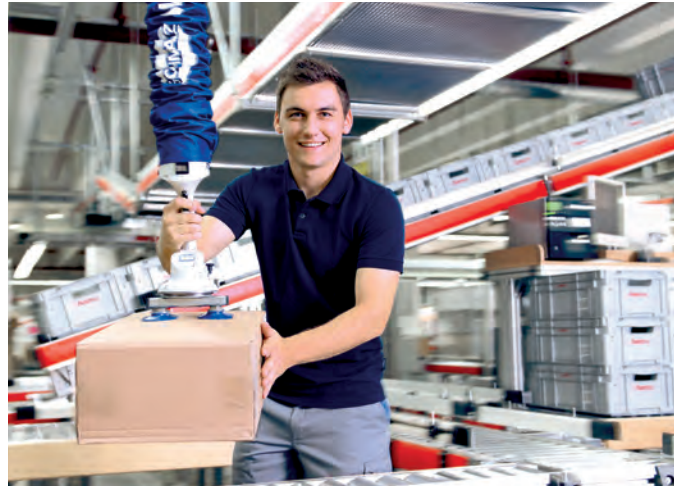
Vacuum tube lifter JumboFlex during commissioning of packages
