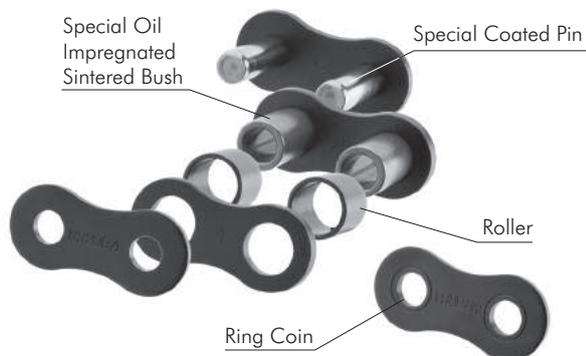
Fig. 23 Basic Construction
