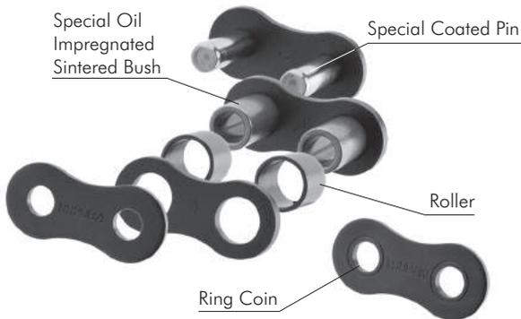
Fig. 22 Basic Construction
