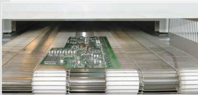
Wire mesh belt used in soldering furnace.
