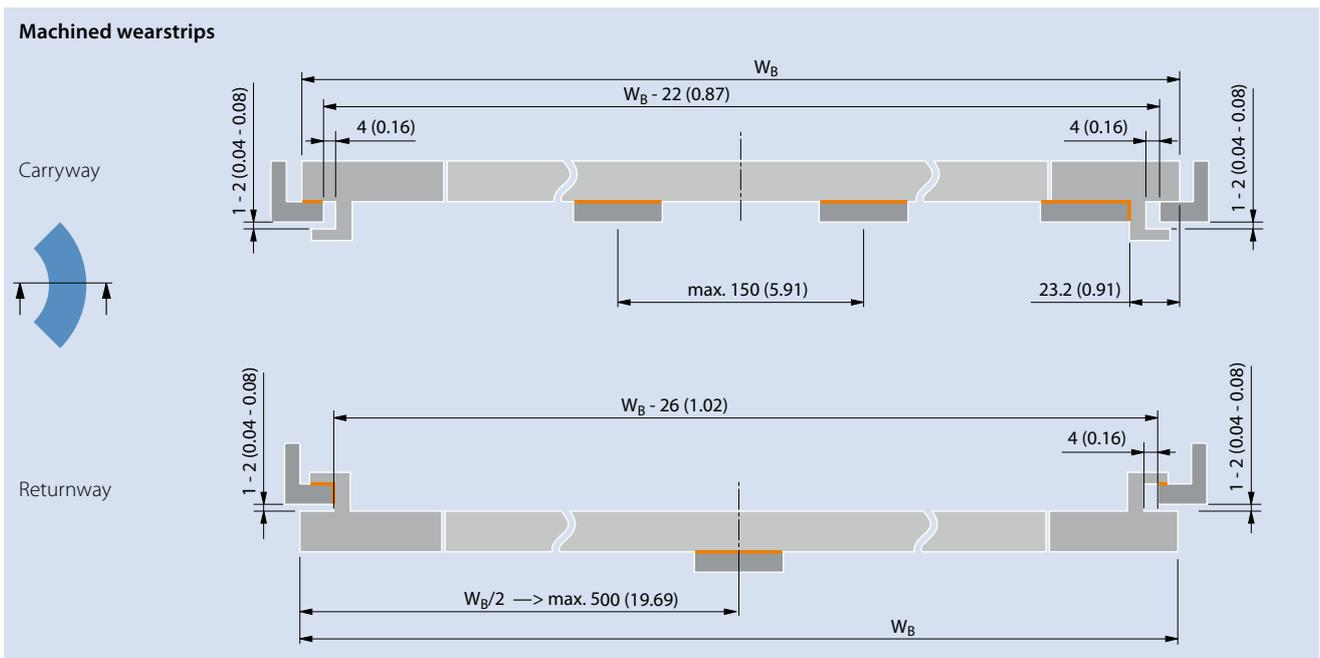
Dimensions in mm and inches (in). All imperial dimensions (inches) are rounded off.
