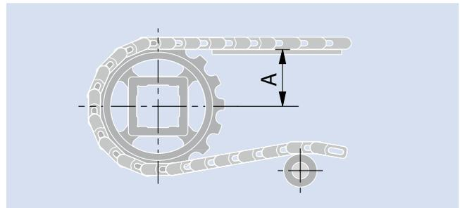
On the sprocket data sheets you find a calculated value for A. The real value will differ slightly due to manufacturing tolerances and temperature-related expansion/contraction, therefore a slight adaption of this value might be necessary to fit your specific needs.
