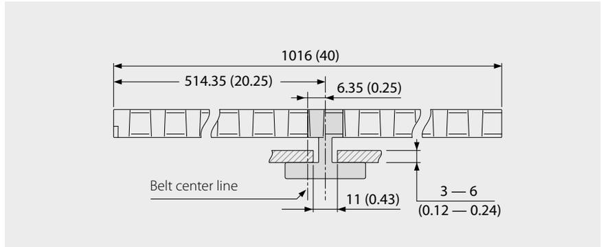
Using Hold Down Tabs results in constraints with regards to sprocket and shaft size to ensure sufficient clearance to the shaft (see also chapter 3.3 hold down tabs).
