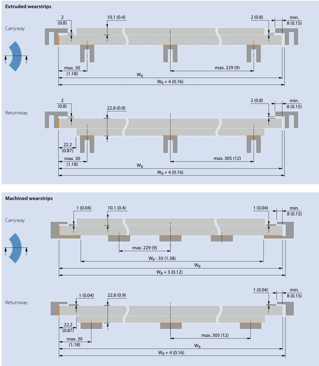
Dimensions in mm and inches (in). All imperial dimensions (inches) are rounded off.
