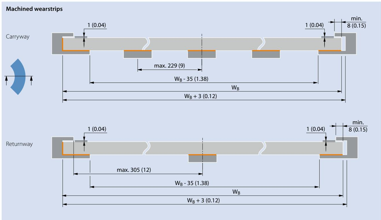
Dimensions in mm and inches (in). All imperial dimensions (inches) are rounded off.
