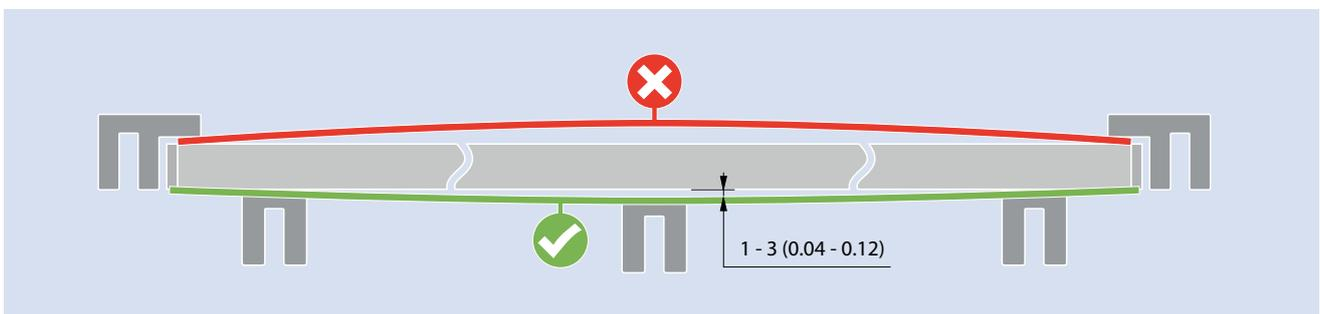
Series 5 and 9 are assembled with steel pins causing a higher stiffness. This reduces the tendency to belt lift in the first place and secondly makes the belt much more laterally stiff
