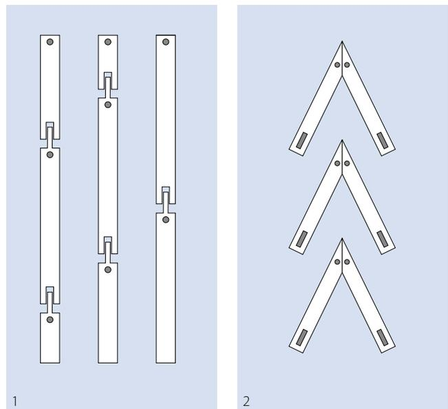
Thermal expansion and contraction must be taken into consideration when mounting the support. These effects can be absorbed by slots and appropriate distancing between the wearstrips (see calculation in "Effect of temperature" in [chapter 4.4](#)). The admissible temperature ranges, as given by the manufacturer, must also correspond to the expected operating conditions.
