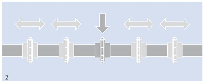
By locking the centermost sprocket equal distribution of belt width expansion and contraction is ensured.
