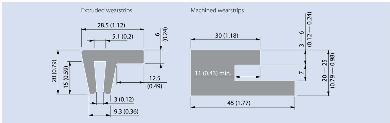
Dimensions in mm and inches (in). All imperial dimensions (inches) are rounded off.
