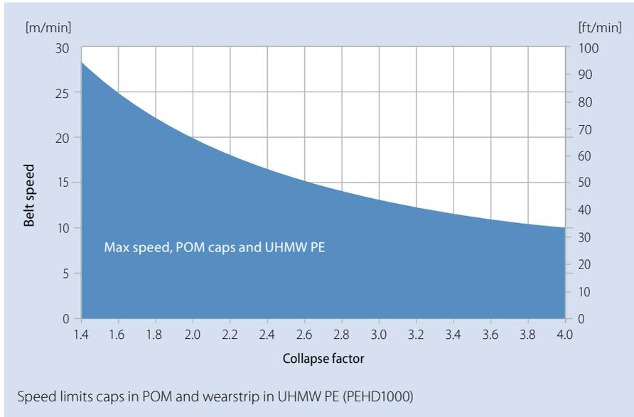
For radius conveyors running at higher speeds, Series 11 offers an alternative with caps or HD on the belt edge made of a special robust, resistant material identified by material code HW. For these we recommend using wearstrips in Nylatron NSM, a special PA material with solid lubricant additives. This material combination will in general offer an extended service life for conveyors with heavy loads or conveyors running in abrasive environments.
