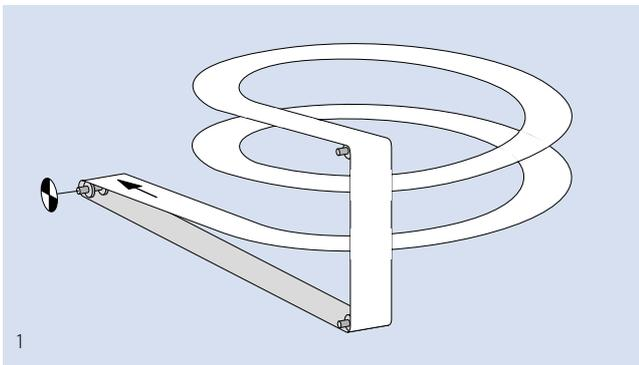
Example of declined conveying to join two production units with different heights (1).
