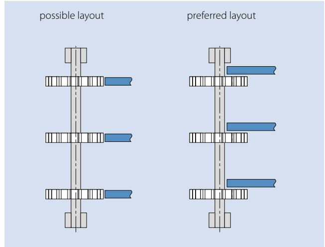
If wearstrips end at the sprocket edge, ensure a distance of  $X \leq 1.5 \text{ Pitch}$ .
