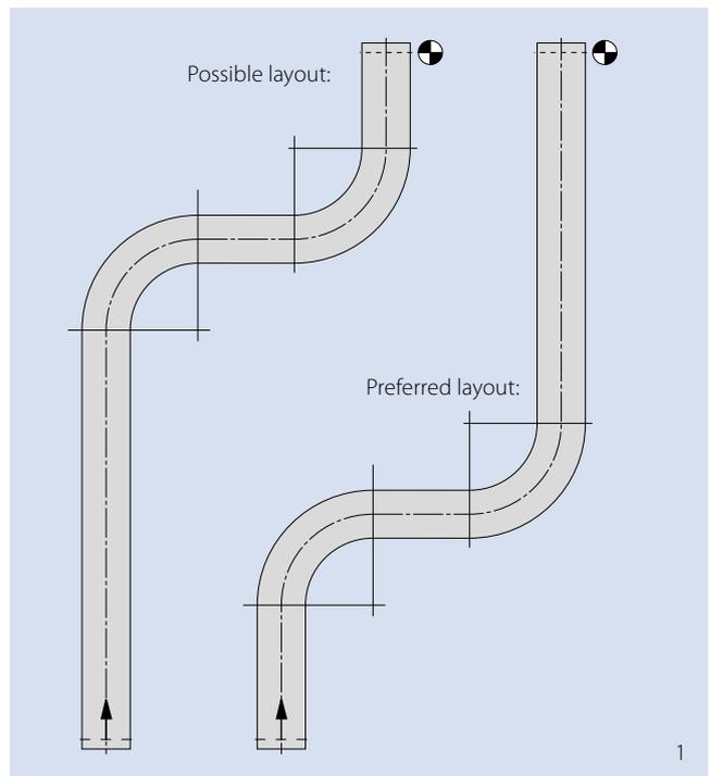
Be aware of a minimum straight section with a distance of one time the belt width before the curve and two times the belt width after and in between curves. This distance in between curves can be reduced if a curve is followed by another one in same direction (2).
