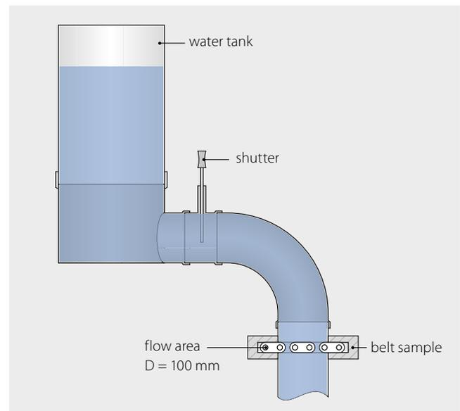
For this reason, Forbo Siegling has developed a drainage test for modular belts. The published “FLOW RATE” is defined in liters per second (l/s) and will support our customer when choosing the right belt for a water drainage application. (Custom testing with other fluids is possible.)
