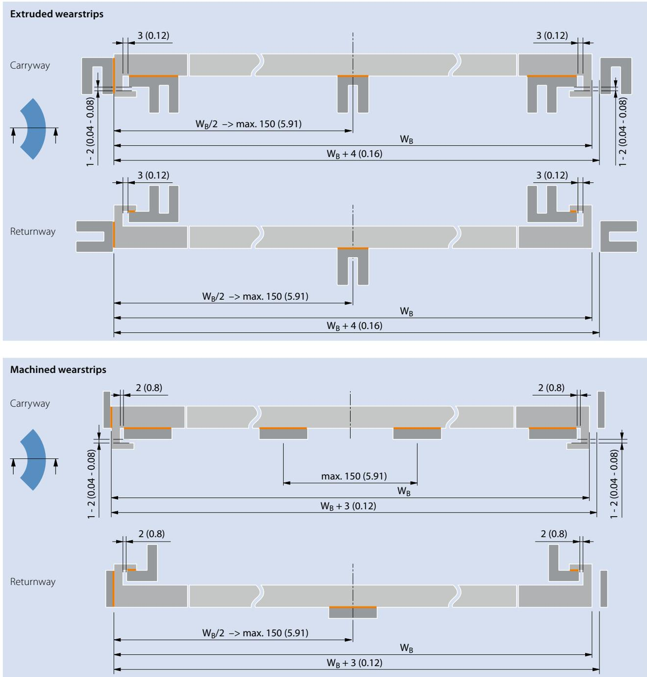
Dimensions in mm and inches (in). All imperial dimensions (inches) are rounded off. Contact areas in orange.
