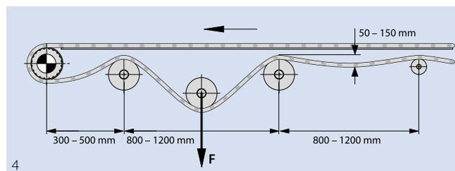
Recommended diameters and weights for conveyor with a center distance up to 10 m (see chart):
