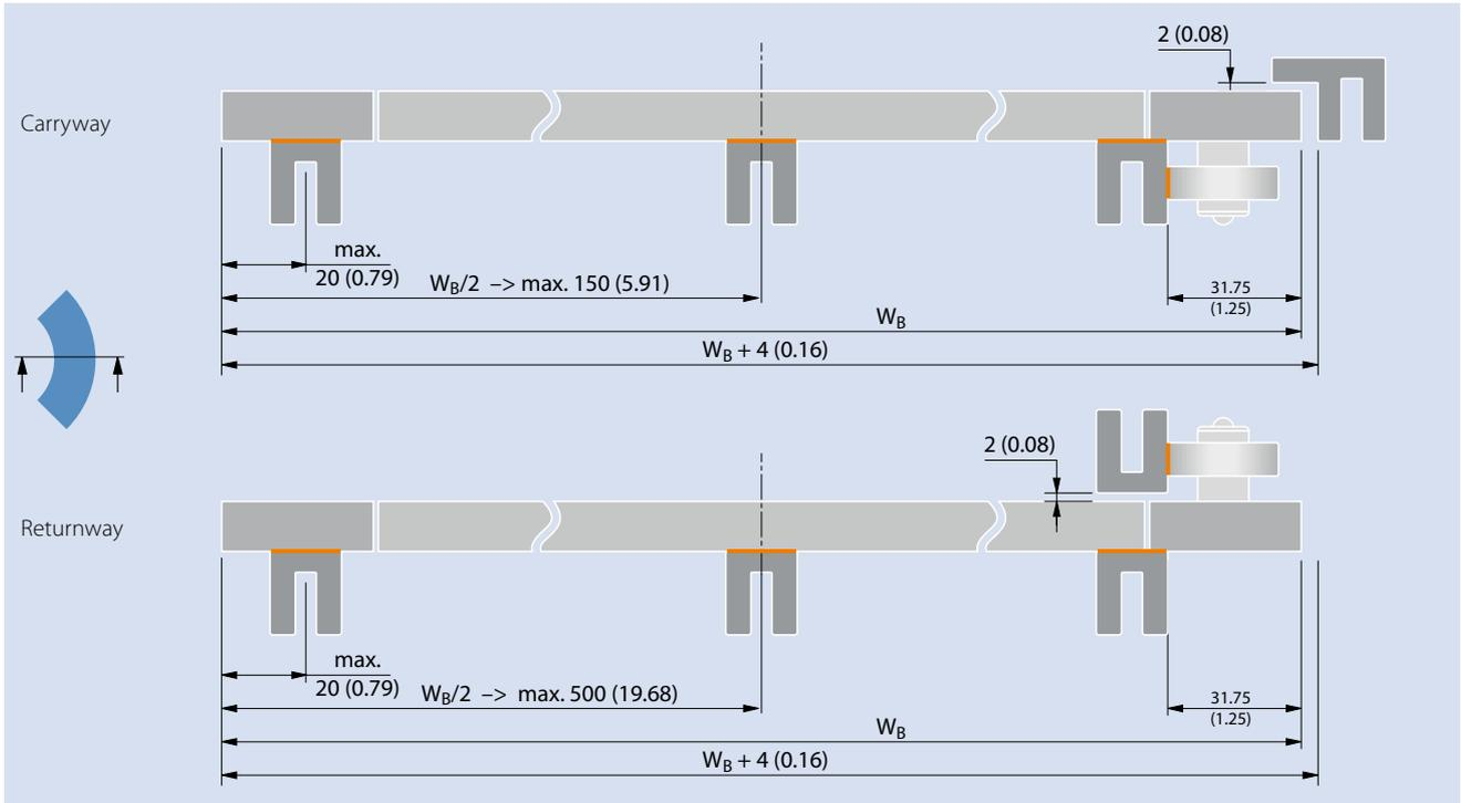
Dimensions in mm and inches (in). All imperial dimensions (inches) are rounded off.
