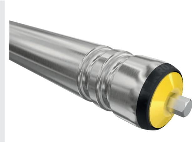
Grooves are running grooves that can be placed in steel or aluminum tubes. They are used to guide round belts. When using the corresponding round belt, they are below the tube surface and, as such, do not contact the conveying good.
