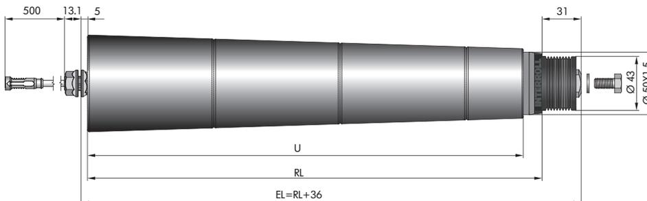
\* Fastening via hexagon spring shaft (shaft not tapered) is not shown here, but it follows dimensional specifications (RL/EL) of the female thread fastening solution shown.
