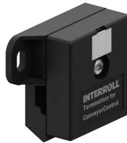
The small termination box serves as terminating resistor for the communication cable of the ConveyorControl system. The termination box can easily contact the cable using piercing technology.
