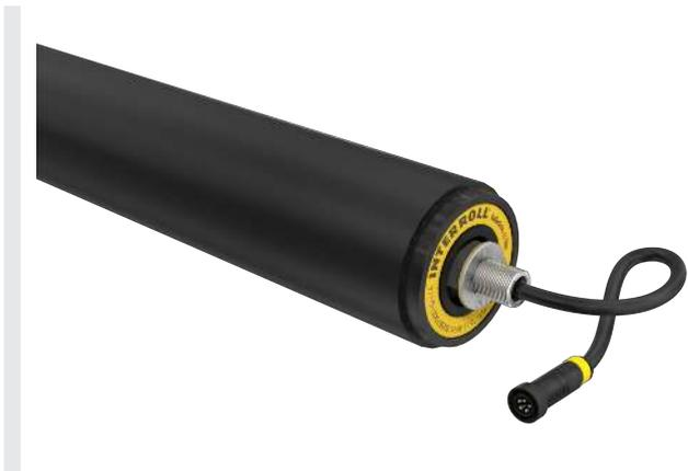
The PU sleeve ensures a high level of noise reduction, particularly for steel containers, and offers a high level of protection of sensitive conveying goods. An improved conveyance of conveying goods is achieved with the higher coefficient of friction compared with a steel tube. Conveying goods can easily be separated since the larger diameter leads to a higher speed with the same rotational speed. With mechanical stress, e.g. with abrasion, it offers a higher robustness than a PVC sleeve.
