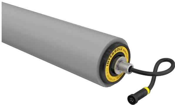
The PVC sleeve ensures a particularly high noise reduction and offers a high level of protection for sensitive conveying goods. An improved conveyance of conveying goods is achieved with the higher coefficient of friction compared with a steel tube. Conveying goods can easily be separated since the larger diameter leads to a higher speed with the same rotational speed.
