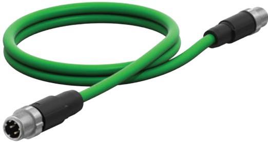
The prefabricated Ethernet cable is used for communication with MultiControl. The cable allows connecting one MultiControl with another MultiControl, another bus node, a switch or a PLC.
