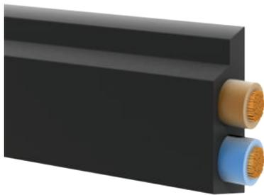
The flat cable is used for the voltage supply of ConveyorControl and MultiControl. The outer contour of the line corresponds to the standard of AS interface. The shell of the line covers holes that were created by piercing contacts. This means that the cable maintains the protection rating even after disconnecting a control.
