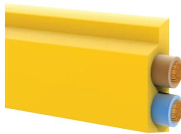
The flat cable is used for the communication of the ConveyorControl control system. The different controls of the system simply contact the line via piercing contacts. The outer contour of the line corresponds to the standard of AS interface. The shell of the line covers holes that were created by piercing contacts. This means that the cable maintains the protection rating even after disconnecting a control.
