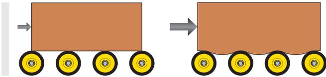
Ribs, keyways, strips or grooves in the bottom of conveying goods that run parallel to the direction of conveyance, do not pose a problem concerning transportability. The required drive output increases depending on their shape. Cross ribs can negatively impact the transporting. It may be necessary to determine the roller pitch empirically.
