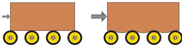
Ribs, keyways, strips or grooves in the bottom of conveying goods that run parallel to the direction of conveyance, do not pose a problem concerning transportability. The required drive output increases depending on their shape. Cross ribs can negatively impact the transporting. It may be necessary to determine the roller pitch empirically.
