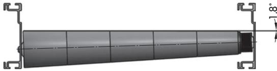
For the curve construction, it must be taken into account that the top side of the curve RollerDrive is level. Hence, the fastening shaft is not horizontal. As a result, vertically arranged side profiles do not have a 90° angle. For this reason, Interroll recommends an angle compensation so that the fastening shaft does not experience any warping. The EC3500 with protection rating IP54 is exclusively available for installation in the curve.
