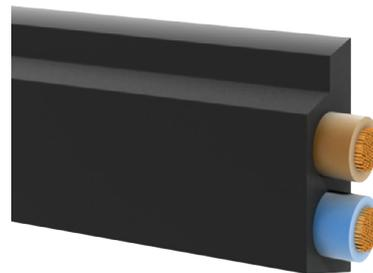
The flat cable is used for the voltage supply of MultiControl. The outer contour of the line corresponds to the standard of AS interface. The shell of the line covers holes that were created by piercing contacts. This means that the cable maintains the protection rating even after disconnecting a control.
