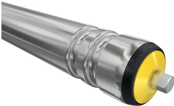
Grooves are running grooves that can be placed in steel tubes. They are used to guide round belts. When using the corresponding round belt, they are below the tube surface and, as such, do not contact the conveying good.
