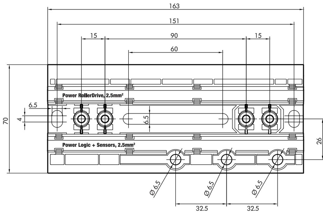
To be able to position the magnetic key, the distance from the top edge of MultiControl to adjacent components must be at least 10 mm.
