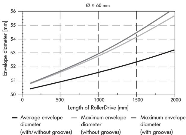
The envelope diameter depicted here only takes into account the tolerances of the rollers and RollerDrive. Tolerances from, for example, installation out of center or tolerances in the grid spacing of the fastening holes are not taken into account.
