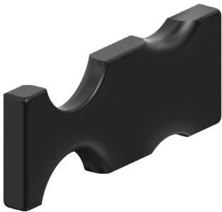
The PolyVee tensioning device enables easy tensioning of 2-rib and 3-rib PolyVee belts and is intended for roller pitches 75 mm and 100 mm. The tensioning device is designed for rollers and RollerDrive with a diameter of 50 mm. It cannot be used for tubes with tube sleeves or tapered elements.
