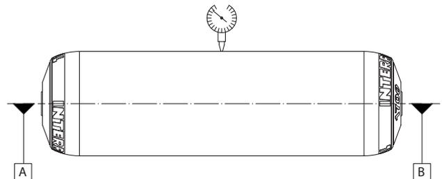
Fig.: Measuring the concentric deviation
