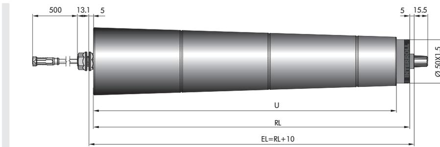
\* Fastening via female thread is not shown here, but it follows dimensional specifications (RL/EL) of the hexagon spring shaft shown.
