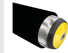
The PU sleeve ensures a high level of noise reduction, particularly for steel containers, and offers a high level of protection of sensitive conveying goods. An improved conveyance of conveying goods is achieved with the higher coefficient of friction compared with a steel tube. Conveying goods can easily be separated since the larger diameter leads to a higher speed with the same rotational speed. With mechanical stress, e.g. with abrasion, it offers a higher robustness than a PVC sleeve.
