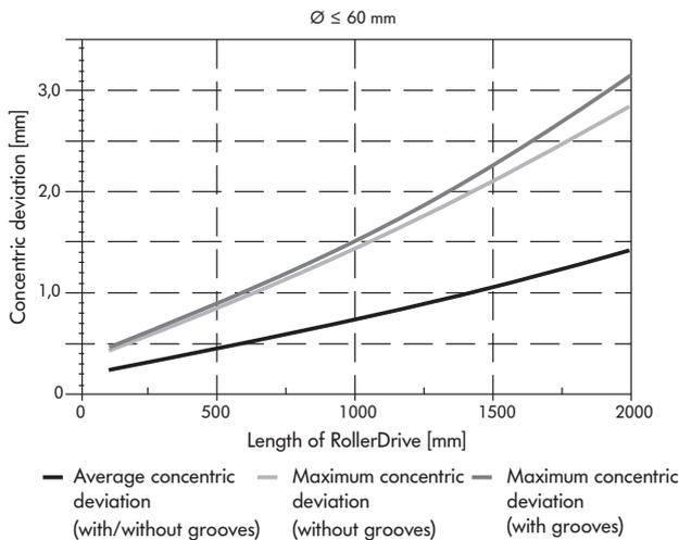
The concentric deviation described above as well as the diameter enlargement due to the integration of grooves result in a theoretical envelope diameter that is larger than the tube diameter. The following diagram shows the respective envelope diameter with respect to the RollerDrive length.
