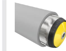
The PVC sleeve ensures a particularly high noise reduction and offers a high level of protection for sensitive conveying goods. An improved conveyance of conveying goods is achieved with the higher coefficient of friction compared with a steel tube. Conveying goods can easily be separated since the larger diameter leads to a higher speed with the same rotational speed.
