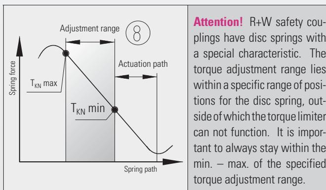
**Attention!** R+W safety couplings have disc springs with a special characteristic. The torque adjustment range lies within a specific range of positions for the disc spring, outside of which the torque limiter can not function. It is important to always stay within the min. – max. of the specified torque adjustment range.
