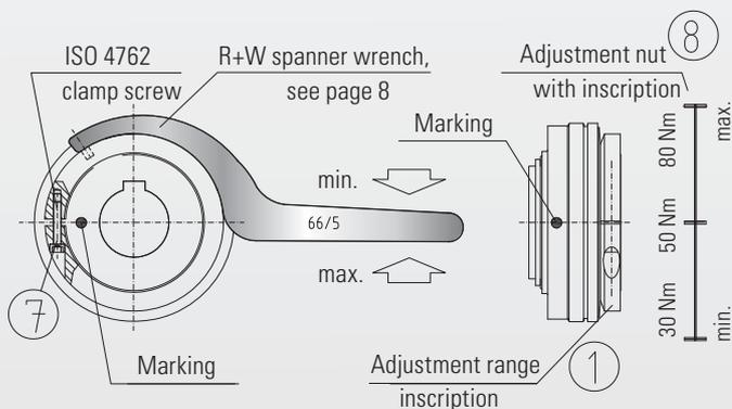
R+W safety couplings are preset and marked with the desired disengagement torque setting at the factory. The min. and max. of the torque adjustment range are then also marked on the adjustment nut (1). Disengagement torque is continuously adjustable within the range (8) through adjustment of the tension on the disc springs.
