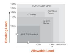
If you've had problems such as fatigue breakage of link plates, or generally poor performance, we recommend that you try the TSUBAKI HT Series, SUPER Series, SEPER-H series or the ULTRA SUPER Series where you can dramatically increase the strength of your chain without having to make major modifications to your existing equipment.
