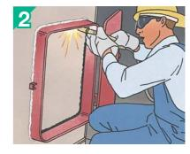
2. Cut the inside hole. Open the door and carefully torch burn the center to create the access area
