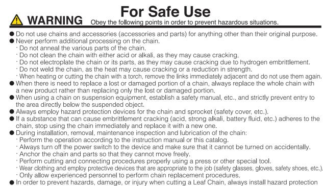
• In order to prevent hazards, damage, or injury when cutting a Leaf Chain, always install hazard protection devices (safety device, etc.) on the suspension equipment employing the Leaf Chain.
