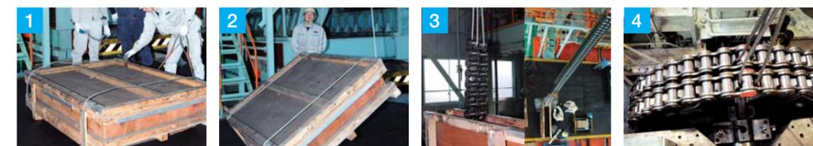
1 Chain is packaged in a special wooden box and delivered horizontally.
