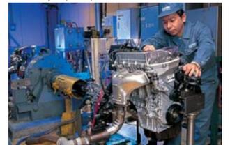
Testing a timing chain drive system
