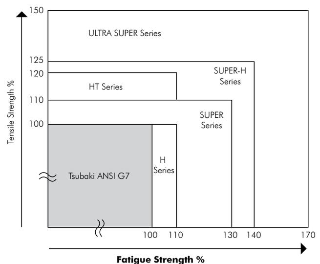
Fig. 16 Comparison of Tensile Strength / Fatigue Strength
