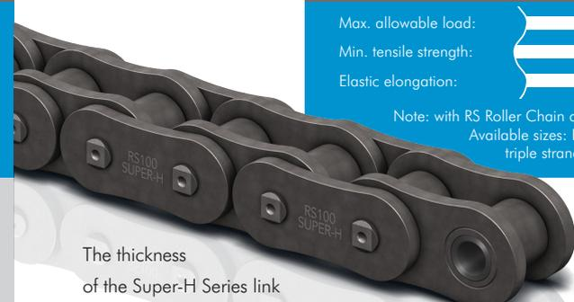
The thickness of the Super-H Series link plates is the same as the next larger pitch size of Super Series chain. The pins are also through-hardened which provides a higher tensile strength and a higher fatigue strength than Super Series chain. The pin holes of the outer link plates are critically formed and ball drifted. The holes of the roller link plates are ring coined to increase fatigue strength.
