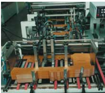
Vacuum-aided discharge of cardboard with perforated Siegling Linpack belts.
