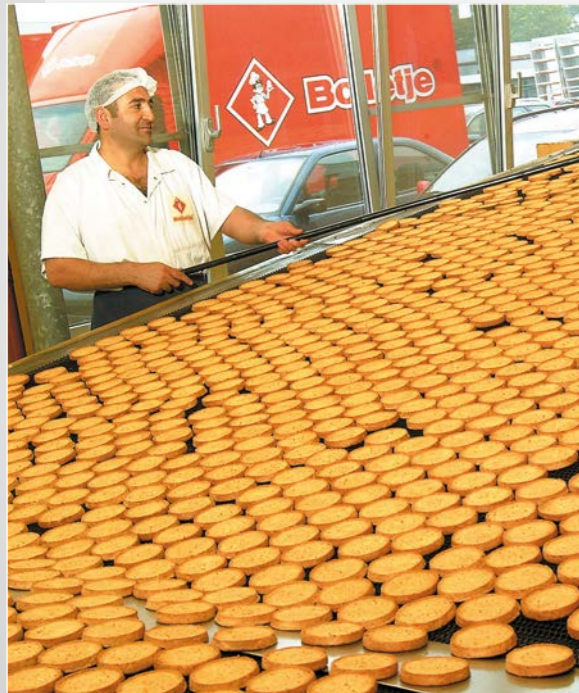
Balanced weave belts are suitable for very heavy as well as very light products.
