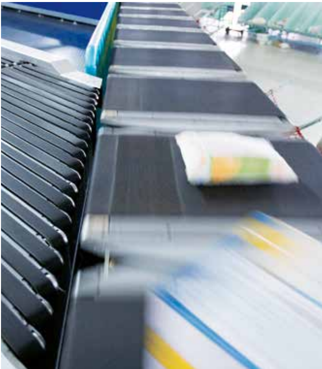
Lateral sorter in a distribution centre. The high acceleration requires the belt surface to have an extremely high coefficient of friction.
