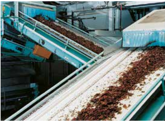
Inclined conveying in the tobacco industry. In this area, conveying angles of up to 22° are possible for belt types with smooth surfaces.
