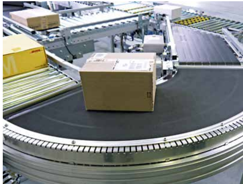
Curved conveyor in a distribution centre.
