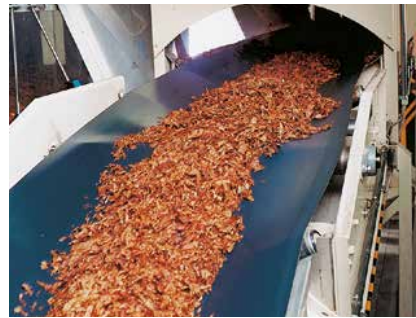
Horizontal conveying with troughable belts. The tension member construction provides the flexibility in the desired direction.
