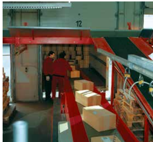
Belts for telescopic conveyors – here being used to unload lorries – must be designed to run with counter bending and at the same time, to withstand high punctual loads.
