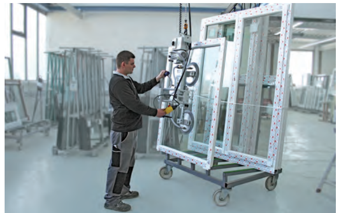
Vacuum lifting VacuMaster Window device being used for picking windows with plastic frames
