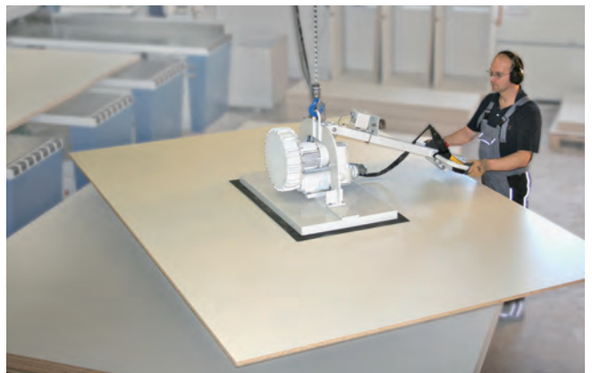
Vacuum lifting device VacuMaster Multi for handling a large, porous wooden board
