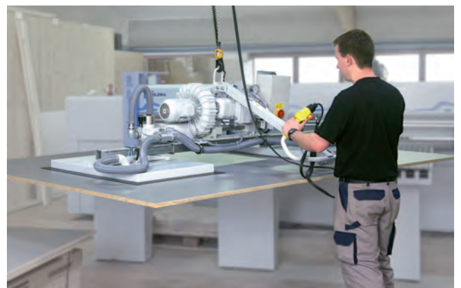
Vacuum lifting device VacuMaster Multi with two suction plates being used to handle heavy, porous wooden boards
