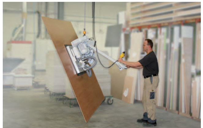
Vacuum lifting device VacuMaster Multi being used to swivel large, porous wooden boards by 90°
