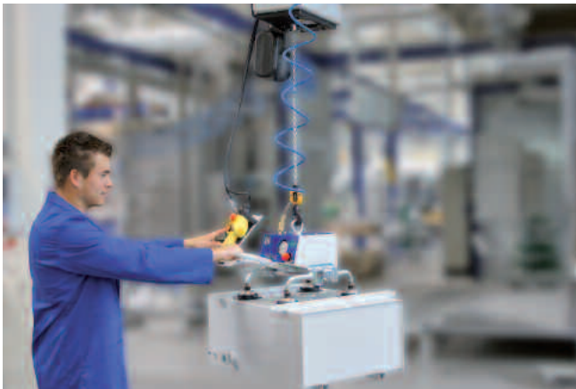
VacuMaster Light, maximum load 100 kg, horizontal, for handling painted furniture elements
