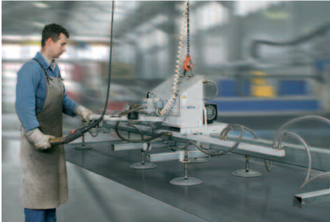
VacuMaster Vario, maximum load 1000 kg, horizontal, for loading and unloading plasma-cutting machines
