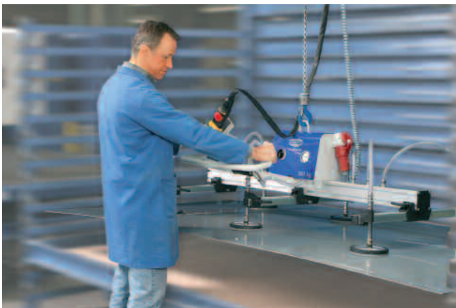
VacuMaster Basic, maximum load 250 kg, horizontal, for loading and unloading sheet metal storage rack systems (more on Page 7)
