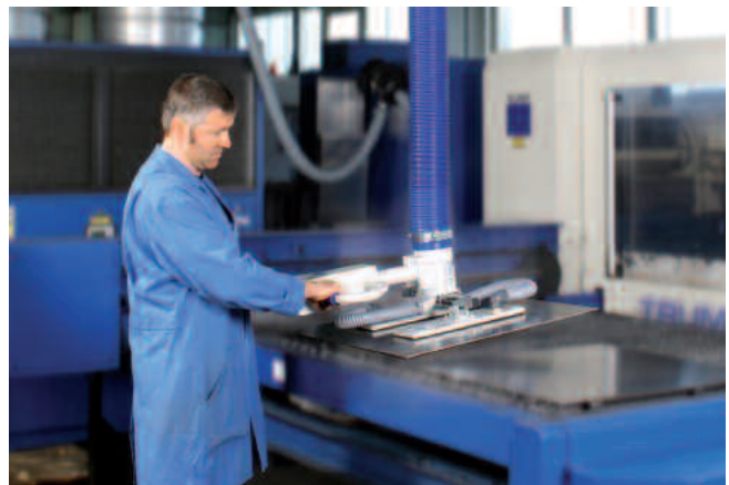
JumboErgo, maximum load 35 kg, with double suction pad FM, for safe movement of raw sheets and machined circular-saw blades (more on Page 6)
