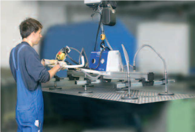
VacuMaster Basic, maximum load 250 kg, horizontal, for handling checker plates (more on Page 7)
