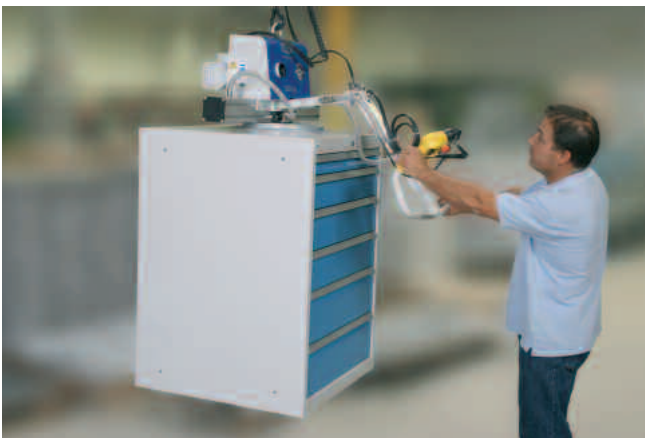
VacuMaster Basic, maximum load 250 kg, horizontal, for handling chests of drawers (more on Page 7)
