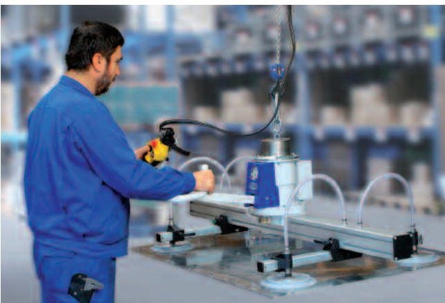
VacuMaster Eco, maximum load 250 kg, horizontal, for handling metal sheets without an external power supply
