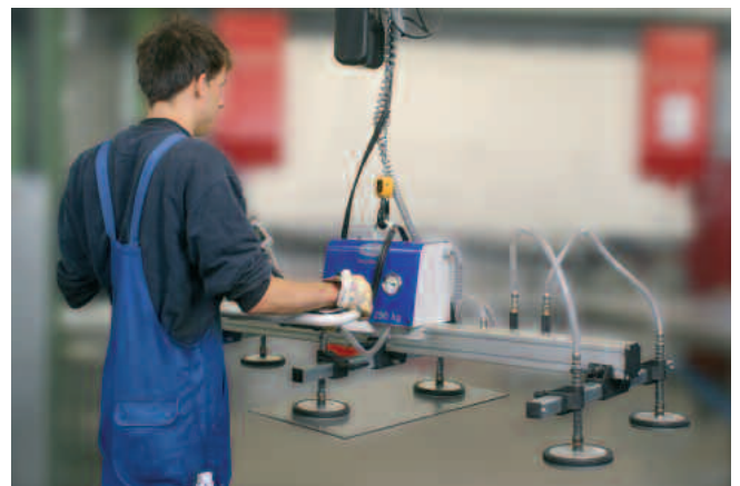
VacuMaster Basic, maximum load 250 kg, horizontal, for handling small metal sheets or sheets with apertures by individual activation of the suction pads (more on Page 7)
