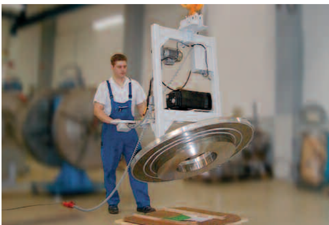
VacuMaster Coil, maximum load 750 kg, with 90° swiveling, for handling of coils
