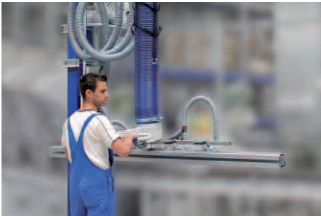
JumboErgo, maximum load 110 kg, horizontal, for handling of aluminum sections (more on Page 6)
