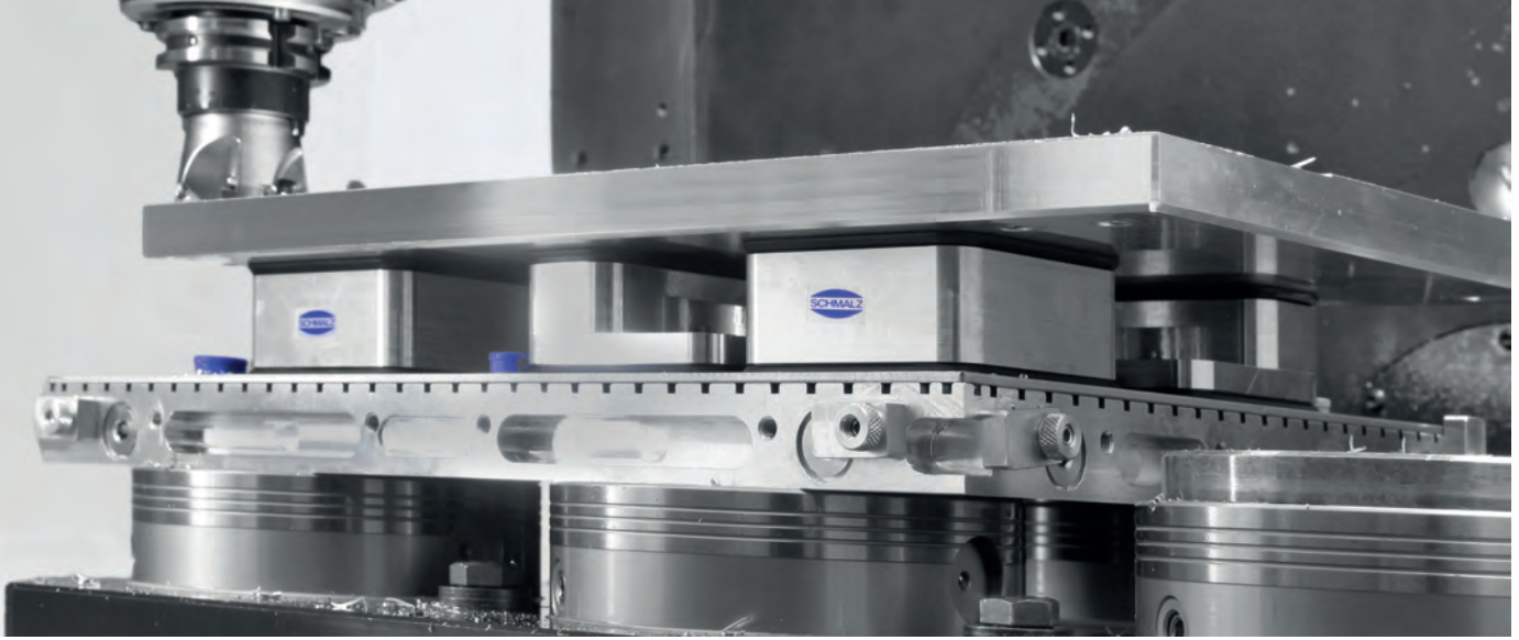
Vacuum clamping system Matrix-Plate with Innospann Steel-Plate and vacuum block for the production of recesses in five-axis processing
