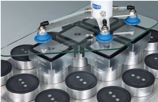
Schmalz Quick-Change System SQC clamping glass components on a Bystronic CNC machining center
