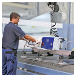
Vacuum lifting devices VacuMaster
