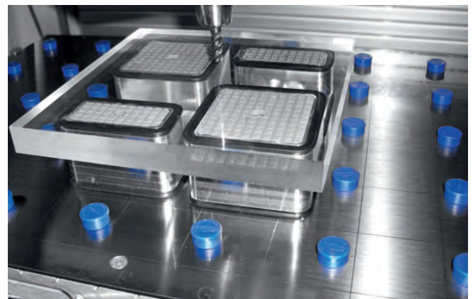
Vacuum clamping system Matrix-Plate with Innospann Steel-Plate and vacuum block, here involved in five-axis processing of a plexiglass plate
