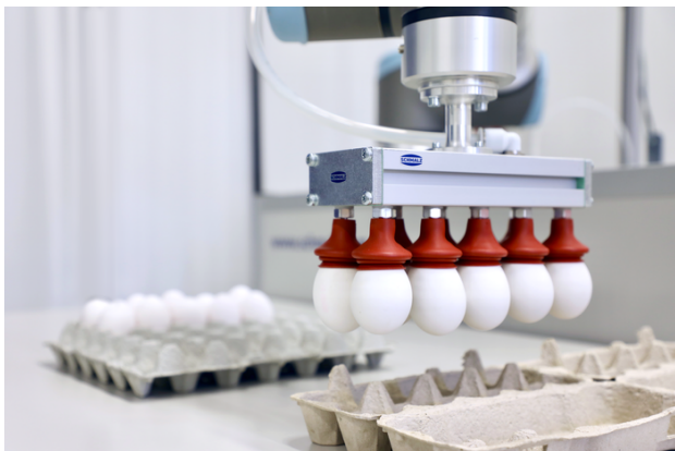
Egg suction cup FG X when handling eggs
