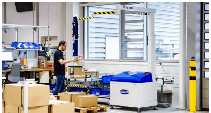
Transportable tube lifter solution JumboFlex Mobile for use in changing locations
