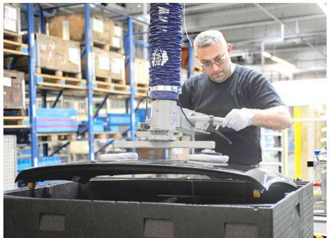
Vacuum tube lifter JumboErgo for handling car body parts
