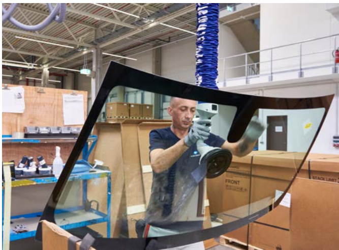
Vacuum tube lifter JumboFlex for handling windshields
