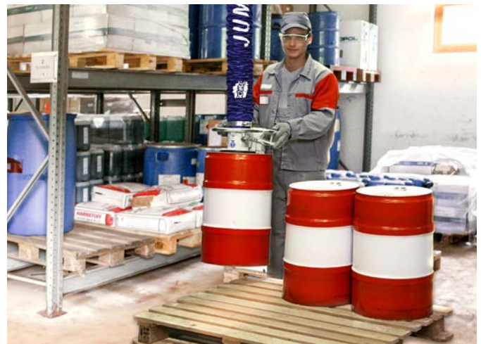
Vacuum tube lifter JumboSprint for handling barrels
