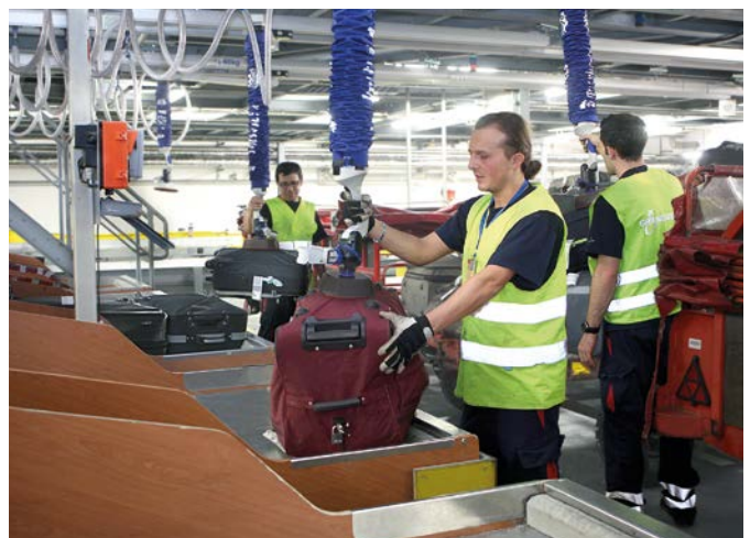
Airport | Vacuum tube lifter JumboFlex for handling of luggage pieces
