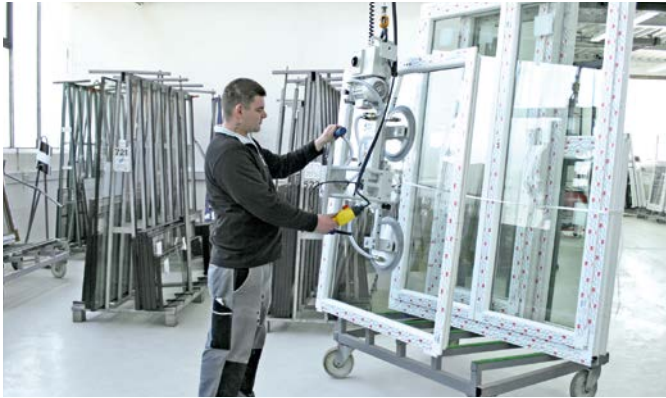
VacuMaster Window for rotating and palletizing windows
