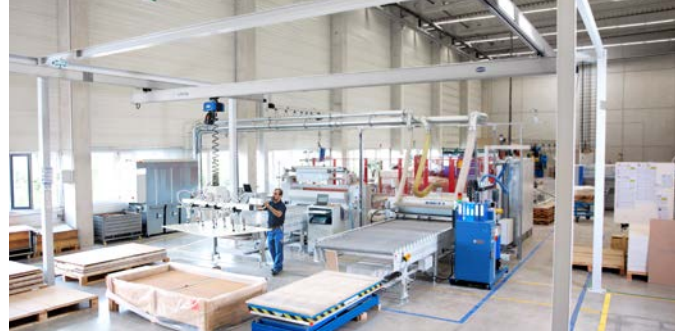
Aluminum crane system SRA with chain host and lifting device VacuMaster
