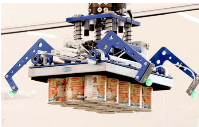
Layer gripping system with pallet clamping and intermediate layer handling for palletizing cans
