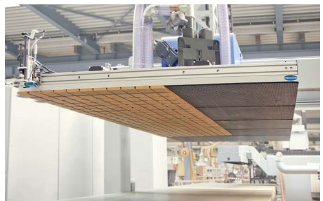
Layer gripping system for de-stacking layers of workpieces in the nesting production
