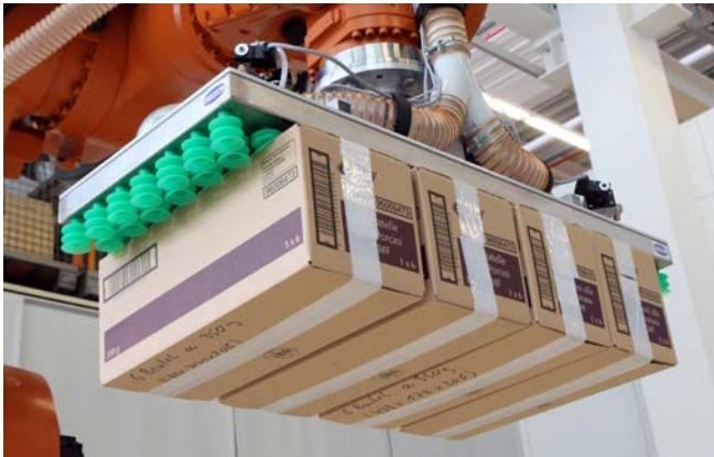
Layer gripping system with suction cups for layer handling of different cardboard boxes
