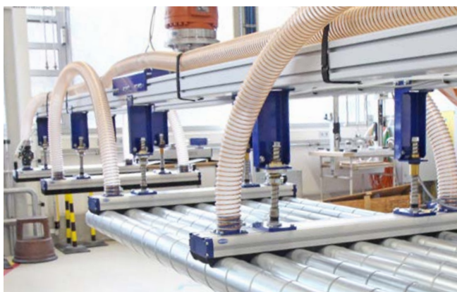
Suction spider with area grippers FMP for handling pipes
