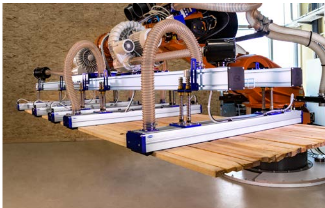
Suction spider with area grippers FMHD for layer by layer handling of rough sawn wooden boards
