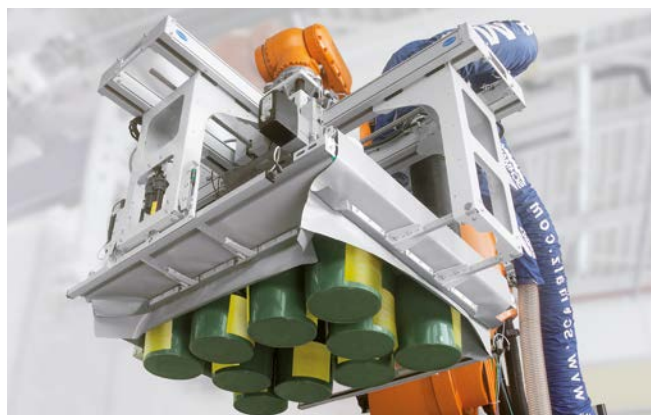
Vacuum layer gripping system SPZ for handling of buckets
