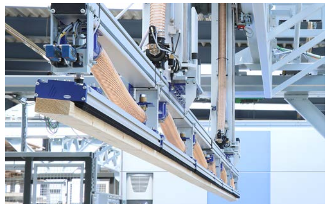
Suction spider with area grippers FMP for feeding a joinery line
