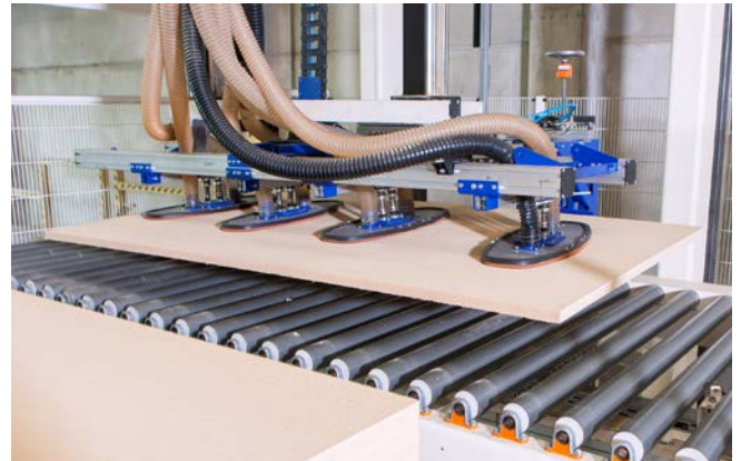
Suction spider with suction plates for handling of porous wood panels
