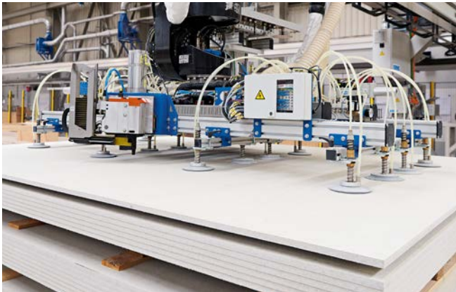
Suction spider with suction plates for de-stacking wooden boards
