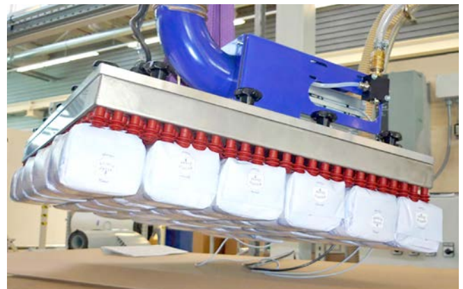
Layer gripping system with suction cups for handling unstable sugar packaging
