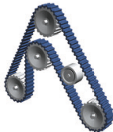
Figure 3.2.2: Multi-pulley drive with inside, smooth cylindrical pulley
