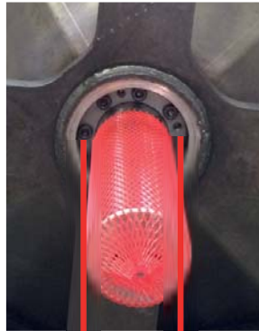
Bar pulley with internal double cone showing
