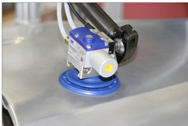
Decentralized vacuum generation by means of ejectors SEAC RP with blow off system right on suction cup
