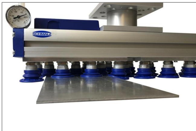
Handling of steel sheets
