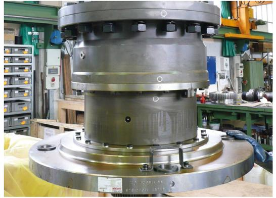
Shear pin type gear coupling
