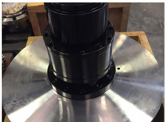
Gear coupling with brake disc.
