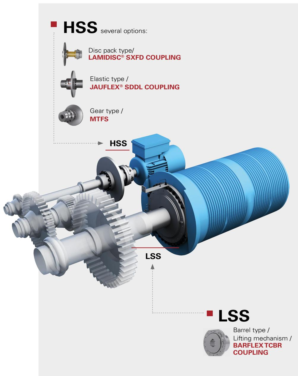
A generalized layout of lifting mechanism is shown in Fig. n° 1. The electric motor shaft is coupled to gear box input shaft by means of high speed flexible coupling, while a TCBR barrel coupling is installed in between gear box output shaft and the cable drum flange.
