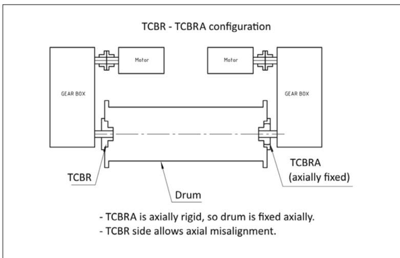
Barrel coupling TCBRA is not designed to support axial load. For each size, there is a maximum value that the coupling can withstand:
