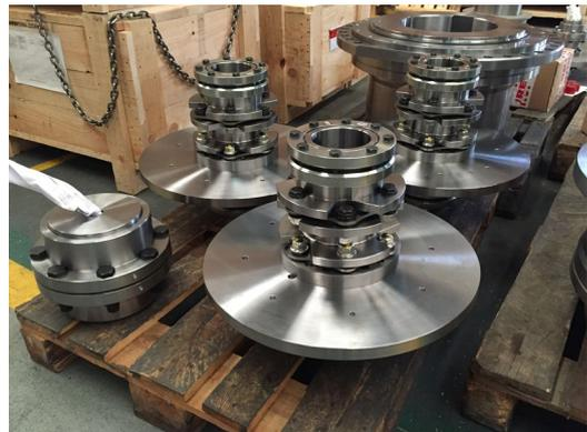
Disc pack configuration with brake disc.
