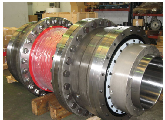
Dredger gear coupling
