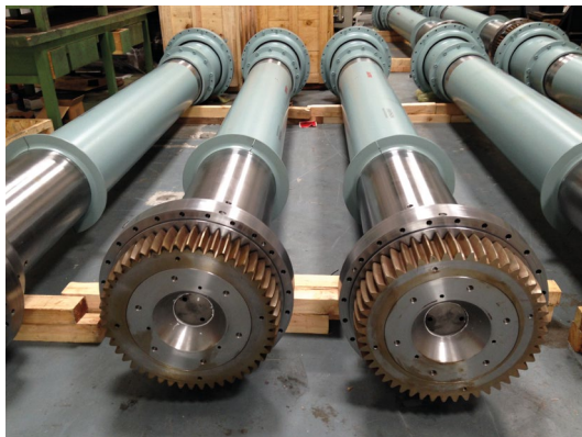
Case carburized gear spindles
