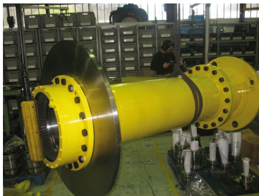
Gear coupling with brake
