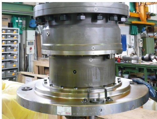
Shear pin type gear coupling
