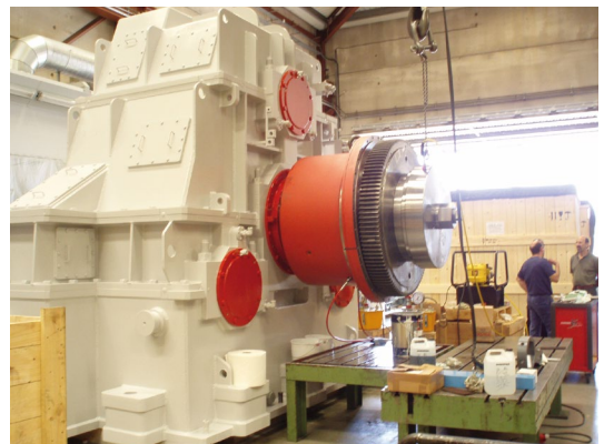
Jaure MTGX-HD-TI-1000 on wind test bench
