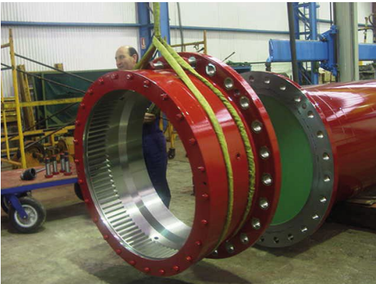
Intermediate gear coupling for HRM
