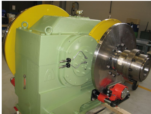
Jaure gear coupling with brake for hoisting
