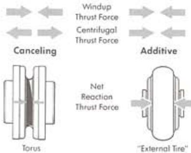
**Less damaging reaction thrust force than external tire types**
