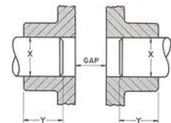
Dimension Y must be equal to or greater than Dimension X for clearance fits, or greater than Dimension X times .75 for interference fits. Example: X = 4" ; the Y must be 4" or more for clearance fits or 3" or more for interference fits.
