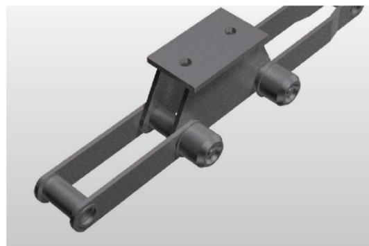
When abrasive material infiltrates between bushes and rollers, and infiltrates outboard rollers, the rollers lock and wear accelerates between bush and roller, causing your chain to reach its wear life. Using TSUBAKI's dust resistant bearing rollers extends the life of your reclaimer chain.
