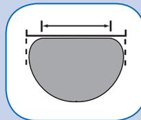
DiaCrimp® wire is precisely shaped to provide the widest flat area possible on top, without increasing the width
