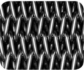
**Gratex belting** – similar to balanced belting except that the spirals are more closely wound, with a straight rod connector, producing a stronger, semi-closed mesh ideal for carrying small parts and heavy loads.
