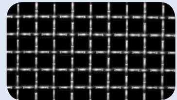
**Lock Crimp** – A securely fixed cloth features deep crimps in the wires at the point of intersection lock the weave. This design of cloth is usually used for heavy-duty screening.
