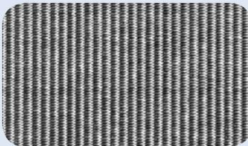
**Twilled Double Dutch** – Similar to Plain Dutch, but twilled weave permits compressing twice as many wires in the same area. The result is maximum density and smooth surface.
