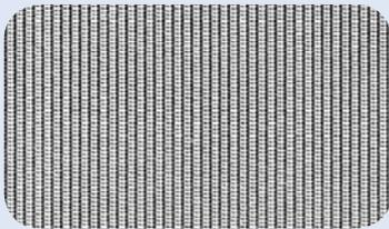
**Plain Dutch** – A compact, firm cloth combining great strength with very small openings. Openings are triangular and positioned at an angle rather than straight up, thereby providing faster and more even buildup of filter cake.
