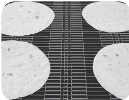
DURAFLEX® offers smooth transport and eliminates product damage during transfer.
