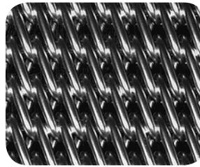
**Duplex belting** – a close mesh with a smooth carrying surface, most efficient for carrying small parts or parts that would be marked by a more open mesh. Woven in pairs of spirals, each pair is turned into the preceding pair and reinforced with a rod through the hinging point, Duplex belting has high strength.
