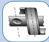
Accurate seating of the diagonally crimped rod maximizes bearing area and stability. Reduced spiral movement
