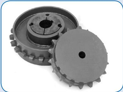
**Machined Steel** – Lasts up to five times longer than cast; concentric; precision machined; cut from solid bar stock; flame-hardened and manually deburred ... and because they're keyed on the centerline of the tooth, they're always matched. Taper lock designs offer easy installation and alignment.
