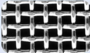
**Plain or Double Crimped** – A general-purpose weave used most often for sizing and straining, or for baskets and assemblies for heat treating processes.
