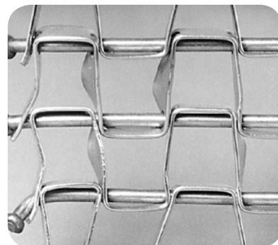
This welded-edge belt is suffering from necking-down, which occurs when the pickets compress on their rods, causing the rods to protrude along the edge. The belt was twisted out of shape when the protruding rods snagged along the edge of the conveyor.
