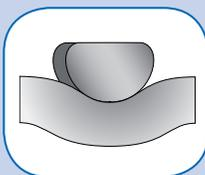
DiaCrimp® is calendared only on the top surface of the spiral, maintaining full curvature on lower surface to better
