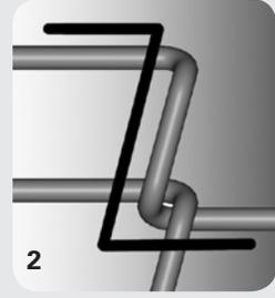
DuraHinge® Belt components (1) are designed with compound angles that hinge at each contact point, reducing stress and maintaining structural soundness. This design also enhances the true tracking nature of the belt.
