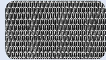
**Oblong** – One of several rectangular weaves that are used primarily for sizing aggregate and similar materials. It provides a greater open area than plain weave, resulting in far less blinding or clogging.
