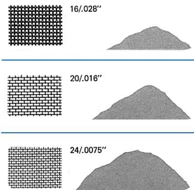
wire sizes provide longer life, but less screened material. Conversely, smaller diameter wires give greater capacity, but shorter service life. The illustrations above demonstrate the relationship between mesh, wire size, open area and screening capacity. ■
