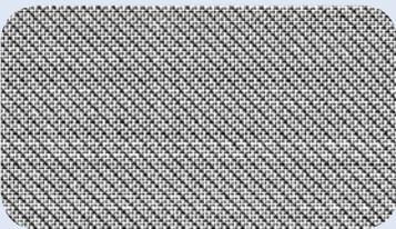
**Twilled** – Permits smaller openings and increased strength as a result of being able to use larger diameter wire.
