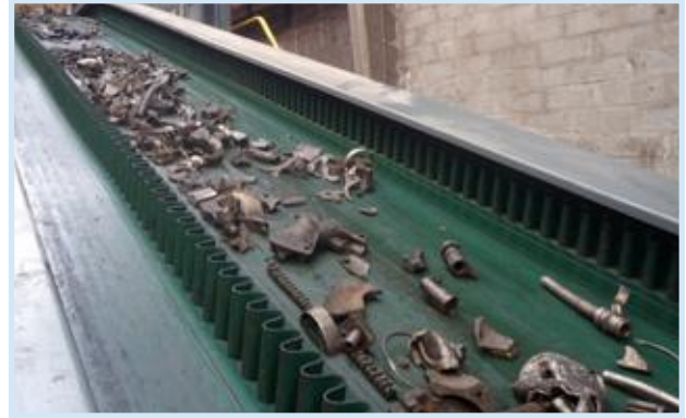
FRZ-5mm with welded Sidewalls: METAL RECYCLING
