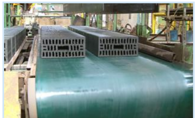
FRZ-4: HEAVY BRICK CONVEYING
