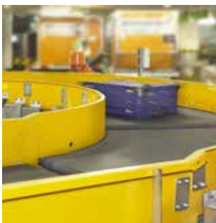
Reliable conveying due to a special fabric structure (distributing forces in the belt well).
