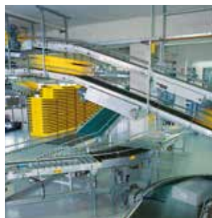
Secure inclined conveying due to conveyor belts with patterns or lateral profiles.
