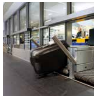
The belts are so flat and smooth that transferring items onto the conveyor from the sides is no problem.
