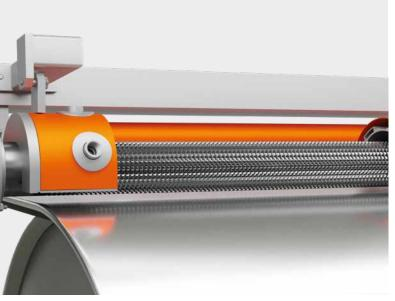
THE MOLTEN PRODUCT IS APPLIED ONTO THE STEEL BELT IN A SHEET FORM USING THE FOLLOWING FEEDING DEVICES. WITH A BREAKER AT THE DISCHARGE END, THE MANUFACTURED PRODUCT SHEET CAN BE SIZED TO THE REQUIRED FLAKE SIZE.
