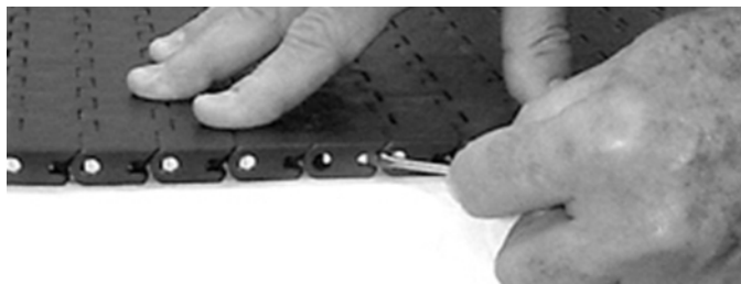
Figure 50: Slidelox rod retention
