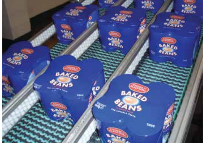
Conveyor with SGDP1505 XP Belt
