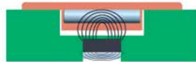
Usual magnetic curve with only 1 magnet
