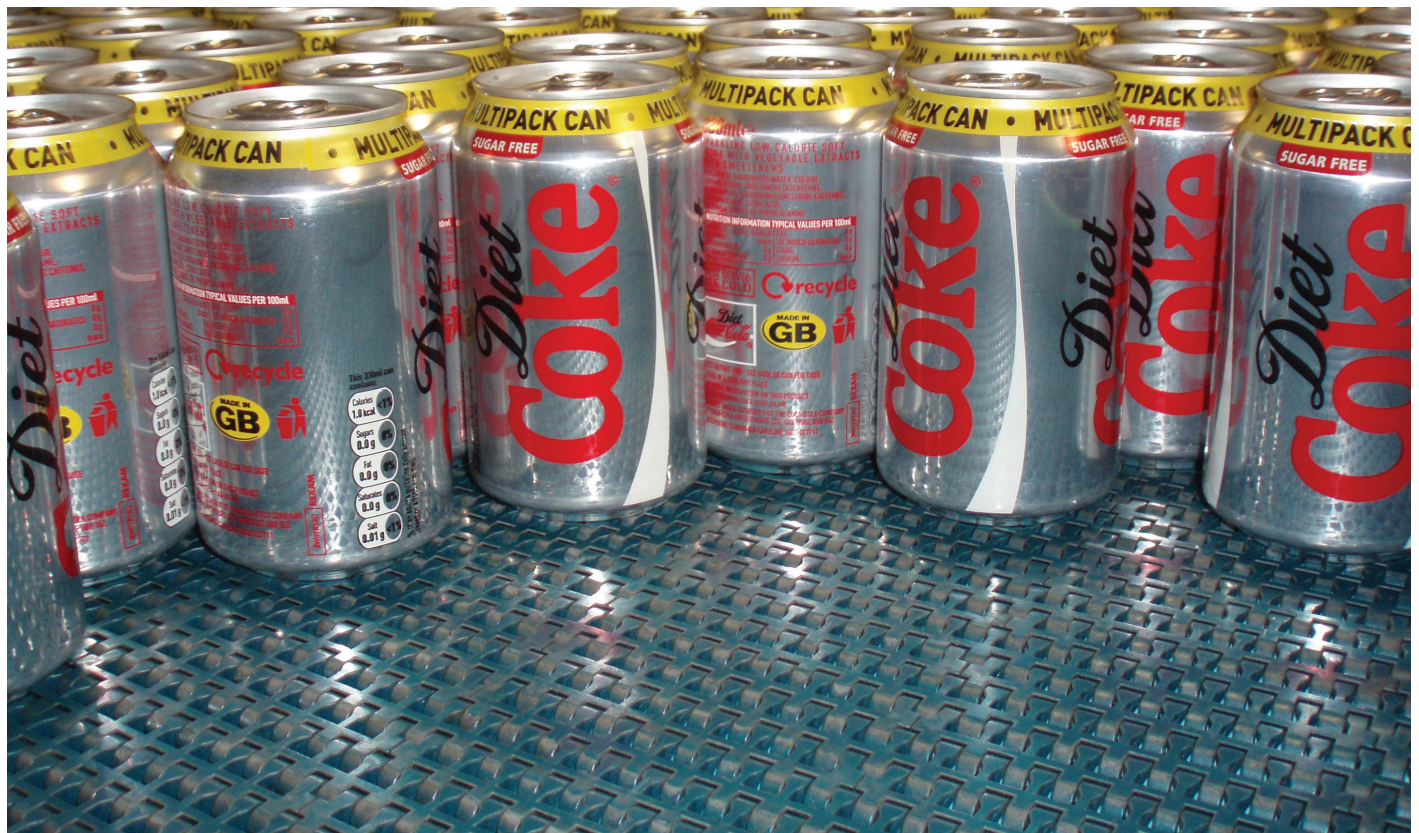
Conveyor with 500 belt.
