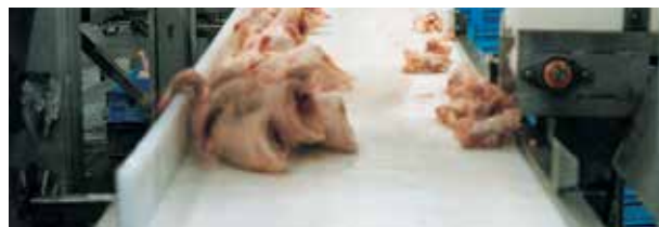
Chicken deboning line with 2015 mattop chain
