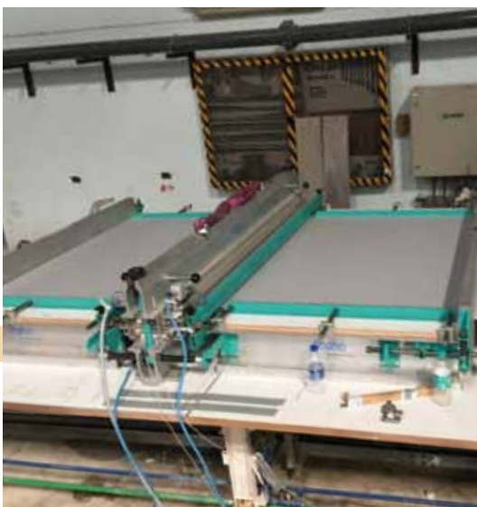
Thursday, 11 a.m. The splice is in the press. Ideal heating settings and control units ensure the splice is strong and leaves no markings.
