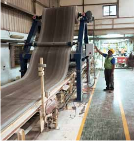
Wednesday, 2 p.m. It's no easy feat, the belt is untensioned, cut, pulled out of the conveyor and wound up.
