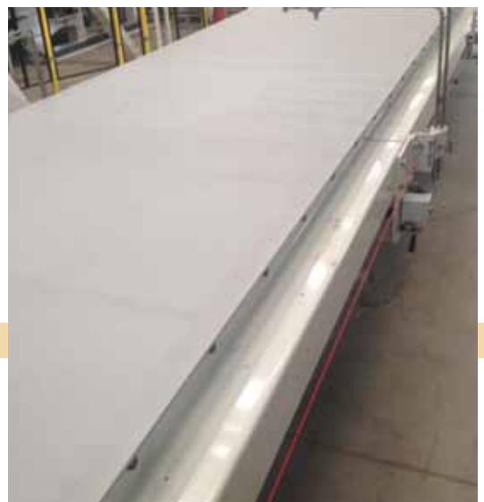
Thursday, 3 p.m. The belt is tensioned and tracked. After inserting the taper edge belts, production can start up again.
