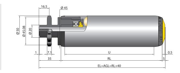
1/2" polymer sprocket head with 14 teeth
