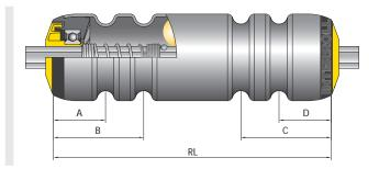
Grooves reduce the concentric precision and load capacity of conveyor rollers. Interroll recommends conveyor rollers with round belt drive heads or PolyVee drive heads of the Series 3500 to ensure that concentric precision is adhered to (page 80).
