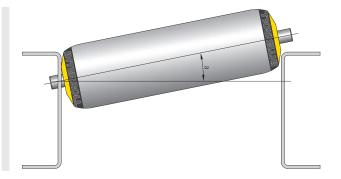
The following formula and the drawings should provide support in sufficiently dimensioning the fastening hole. For this purpose, an oversize of 0.5 mm of d1 compared to the shaft diameter is sufficient in most cases. In case of side profiles with different heights, the dimension H of the higher profile must always be used for the calculation.
