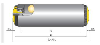
Example: At the time of ordering, a lane width (EL = installation length) of 500 mm is specified for a roller of series 1700 with female threaded shaft. The dimension from seal to seal measures approx. 499 mm. Hence, the roller has an axial play of approx. 1 mm (see figure above).
