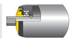
Flatted shafts are made of round material. They have two lateral, parallel milled sections at the shaft ends, which fit into corresponding side profile holes, e.g. into side profiles with open longitudinal holes.
