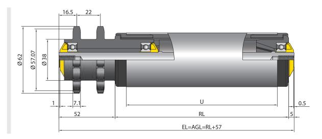
Double friction conveyor roller
