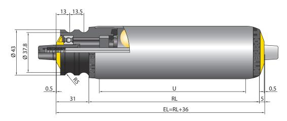
**ROLLERS SERIES 3500** Fixed drive conveyor roller
