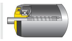
Conveyor rollers must not be warped during installation or operation. This means that play must exist between the seal of the roller and the side profile. The roller must move in axial direction under load.
