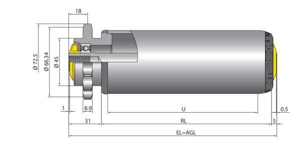
Welded 5/8" steel double sprocket head with 13 teeth
