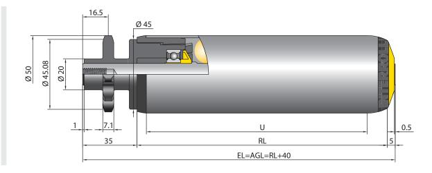
**ROLLERS SERIES 3500** Fixed drive conveyor roller
