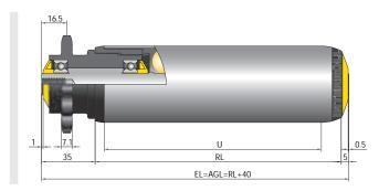
The axial play under consideration depends on roller series and roller version. For example, an axial play of approx. 1 mm on the drive side and 0.5 mm on the other side is taken into account for a roller of series 3500 with sprocket head (see figure above).
