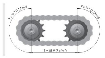
The following theoretical pitches (measured at the sprocket with a pitch of 1/2" and 14 teeth) have been proven and tested:
