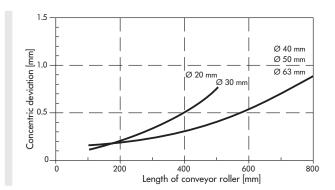
For steel tubes  $\leq 2$  mm wall thickness, Interroll offers a 100% check. In the process, the concentric precision of every roller ordered is checked and, if needed, the tube is straightened. Carbonitrided tubes cannot be straightened.
