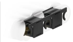
The PolyVee tensioning device enables easy tensioning of 2-rib and 3-rib PolyVee belts and is intended for roller pitches 75 mm and 100 mm. The tensioning device is designed for rollers and RollerDrive with a diameter of 50 mm. It cannot be used for tubes with tube sleeves or tapered elements.
