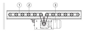
With wrapped force transmission, every conveyor roller is connected to the next one by a chain (1). For this reason the conveyor rollers require double sprocket heads (2). They need more space than with a tangential drive, so that the installation length of the roller is longer. Double sprocket heads always feature a DIN gearing (standard gearing).
