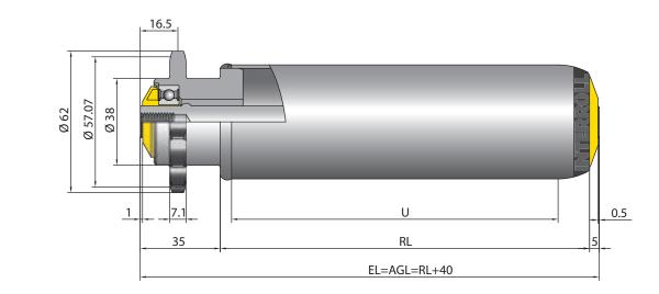
Welded 1/2" steel double sprocket head with 14 teeth
