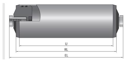
Slide bearing conveyor roller
