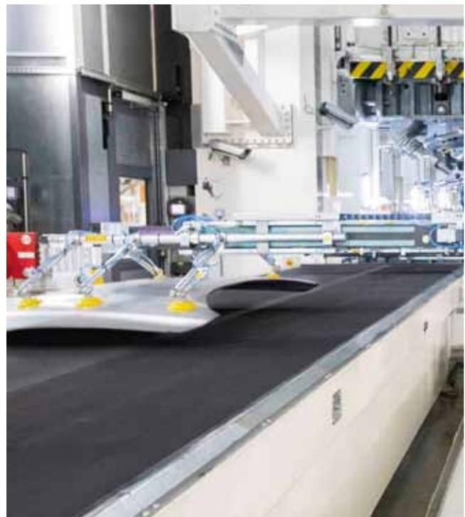
Particularly abrasion- and incision-resistant Siegling Transtex belts guarantee reliable conveying in assembly feed and sheet metal manufacture.
