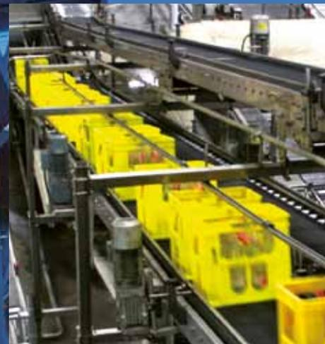
Large gradient angles can be achieved even for heavy-duty loads and when products conveyed are wet.
