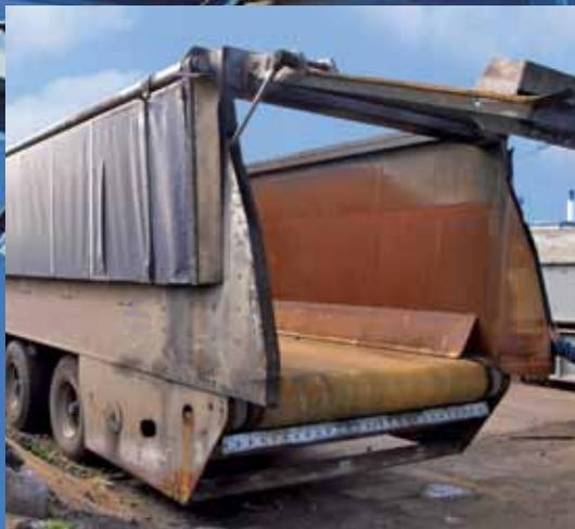
Unloading belt for 40 tons of hard coal. It took Siegling Transtex to make this compact conveyor design possible.
