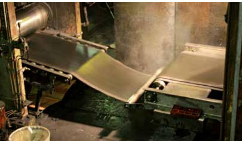
After rolling, 160°C hot rubber sheets are immediately transferred to highly temperature-resistant Siegling Transtex belts.
