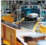
Perfect transfer of items conveyed due to small return radii; short take-up ranges thanks to the belts' tight length tolerances.
