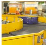
Reliable conveying due to a special fabric structure (distributing forces in the belt well).
