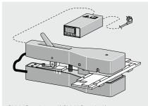
SM-HC-50/40 and SM-HC-80/60 heating clamp for the E line (Z-splice, splice length 70 mm and 35 mm)
