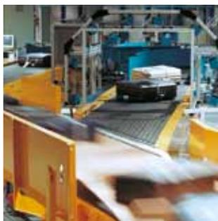
Perfect transfer of items conveyed due to small return radii; short take-up ranges thanks to the belts' tight length tolerances.
