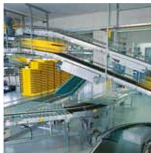
Secure inclined conveying due to wide conveyor belts with patterns or lateral profiles.
