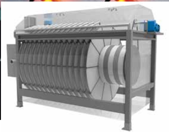
Tertiary Water Filtration
