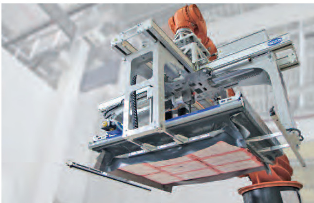
SPZ Logistics | Handling of various product layers in warehousing and intralogistics
