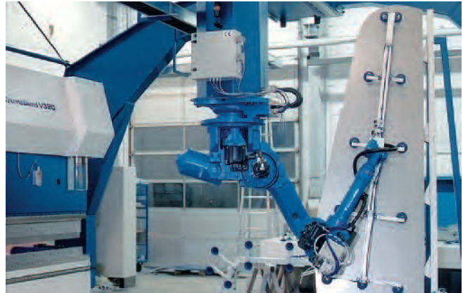
Vacuum suction spider SSP being used to handle cut metal sheets
