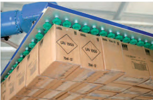
Vacuum layer gripping system SPZ for handling cardboard boxes in layers
