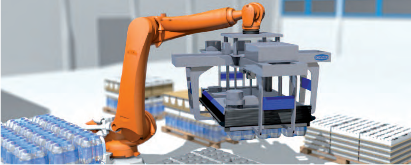
Vacuum layer gripping system SPZ-M-C for palletizing and de-palletizing a wide range of goods
