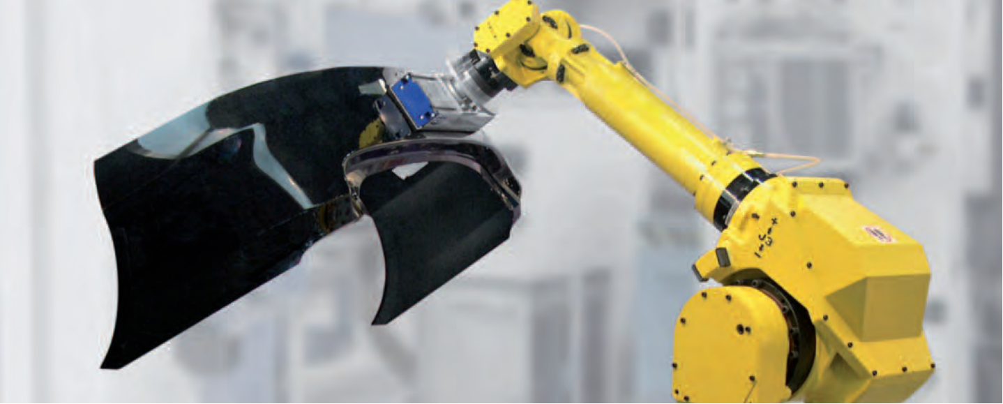
Vacuum area gripping system FXP being used to handle plastic bumpers
