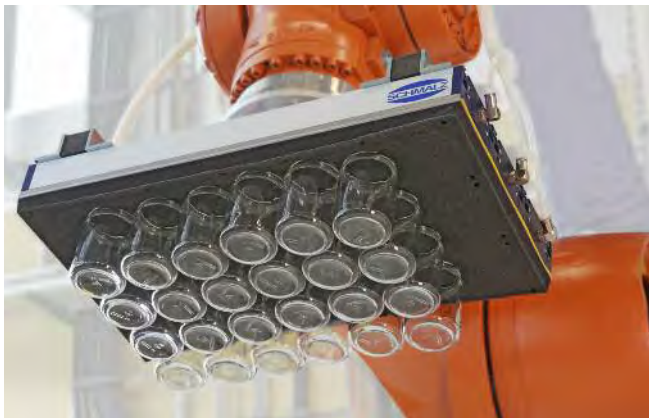
Vacuum layer gripping system SPZ for handling empty jars
