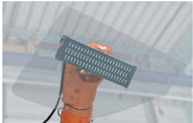
Vacuum area gripping system FXP being used to handle automotive glass during vehicle assembly
