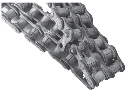
Corrosion of stainless steel drive chain
