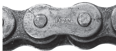
Hydrogen embrittlement cracking
